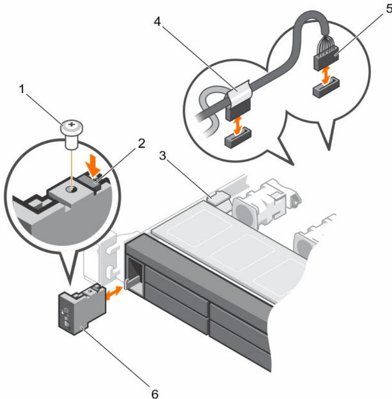
**Figure 53. Removing and installing the control panel—ten 2.5 inch hard-drives/SSDs chassis**
