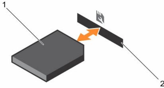
**Figure 34. Removing and installing the SD vFlash media card**
