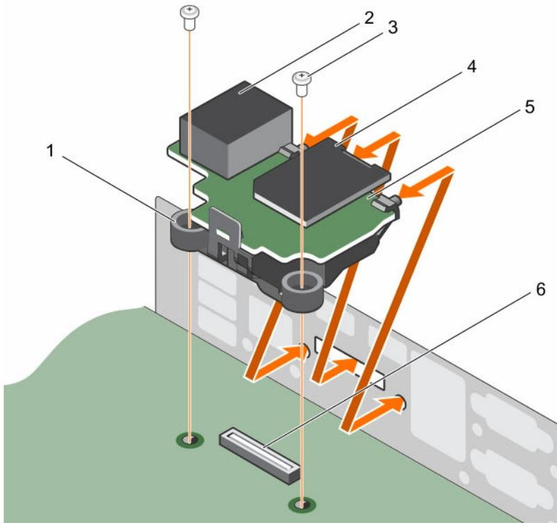
**Figure 33. Removing and Installing the iDRAC port card**
