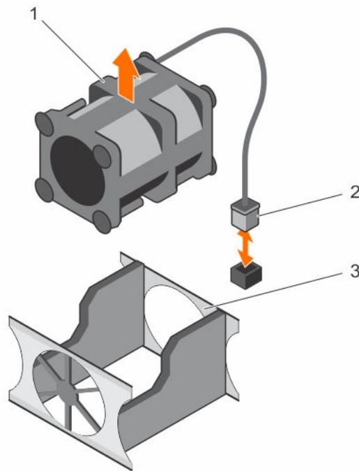
**Figure 29. Removing and installing a cooling fan**
