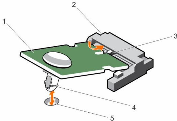
**Figure 59. Installing the TPM**
