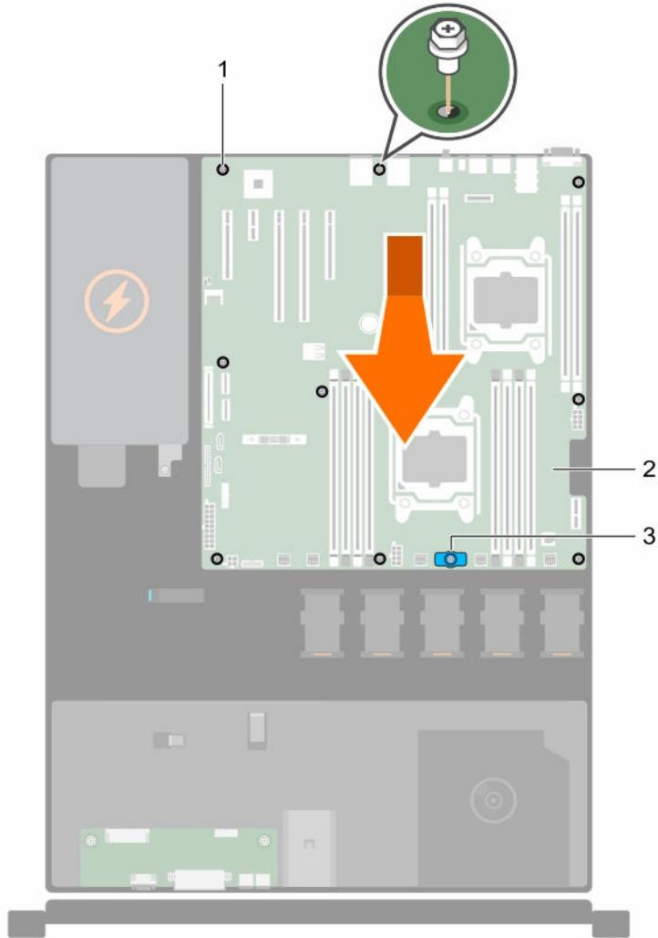
**Figure 58. Removing and installing the system board**
