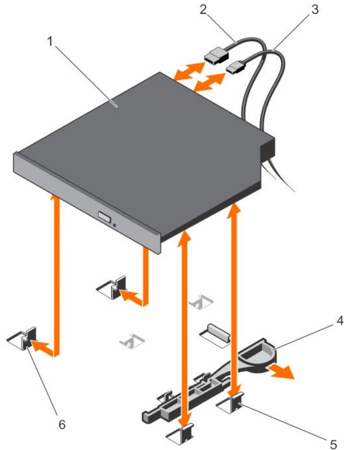
**Figure 28. Removing and installing the standard optical drive**
