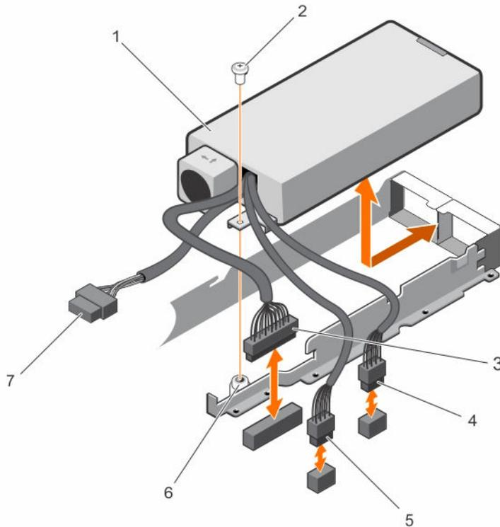
**Figure 42. Removing and installing a non-redundant power supply**
