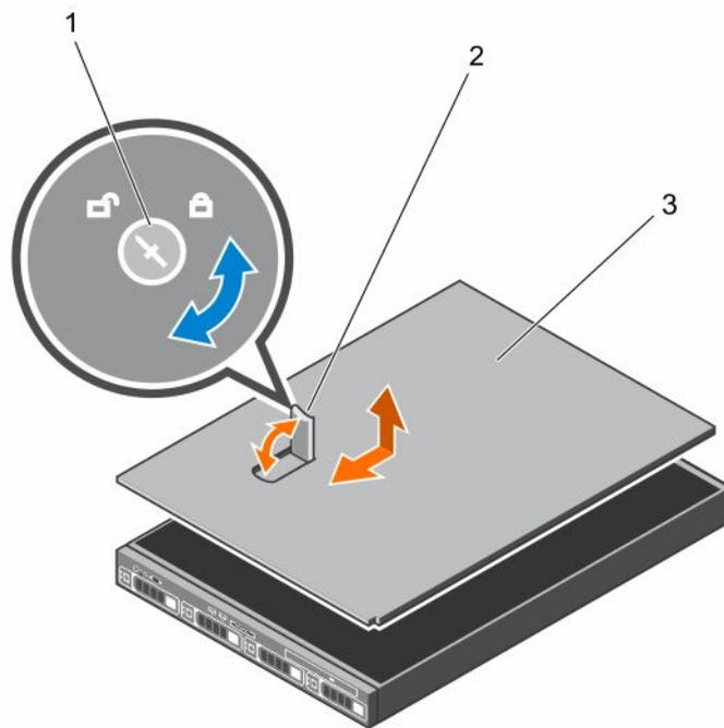
**Figure 13. Removing and installing the system cover**
