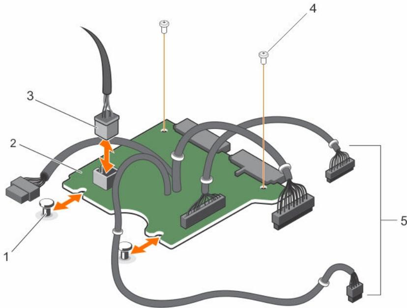
**Figure 57. Removing and installing the power interposer board**
