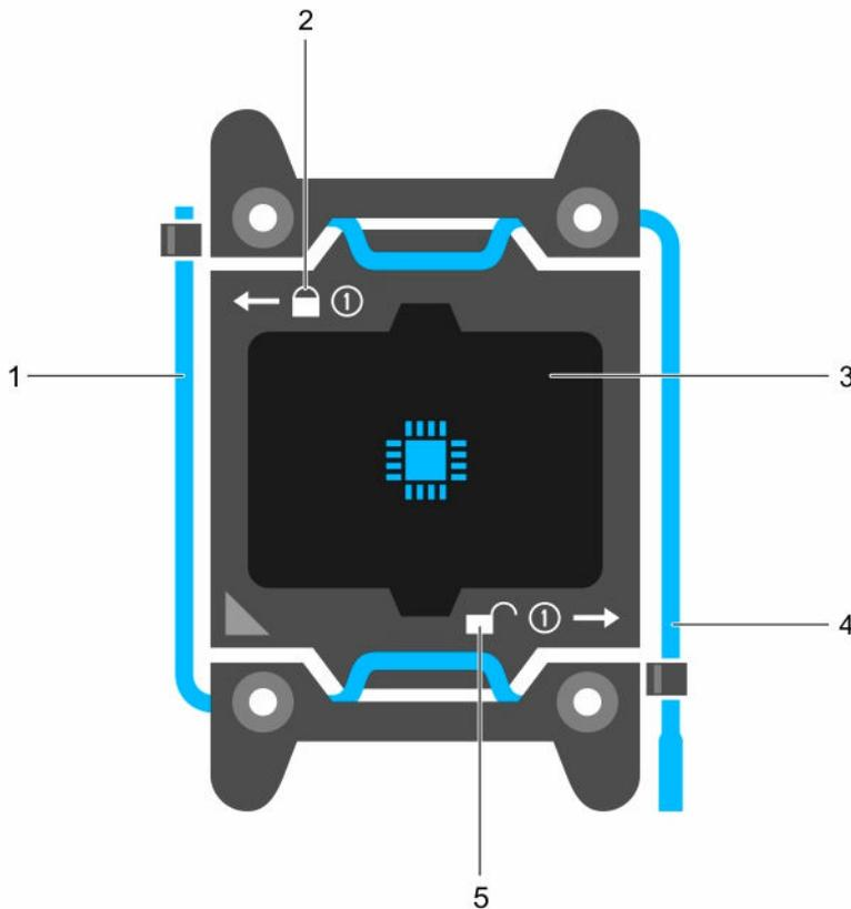
**Figure 37. Processor shield opening and closing lever sequence**
