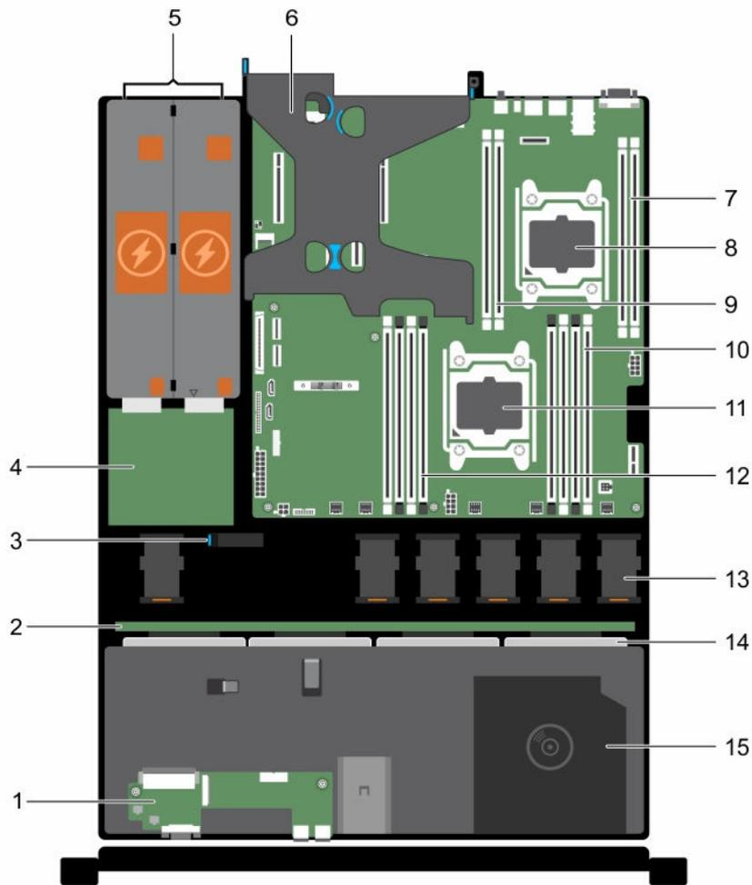
**Figure 15. Inside the System—with redundant power supplies**
