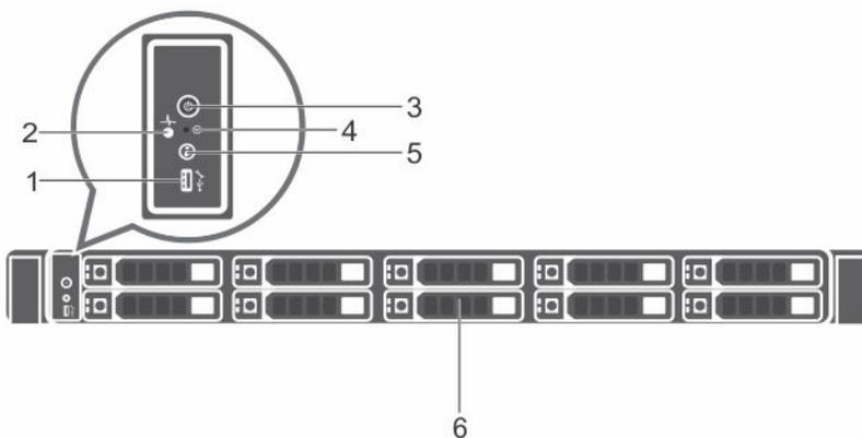
Figure 3. Front-panel features and indicators—ten 2.5-inch hot-swappable hard-drives or SSDs chassis
