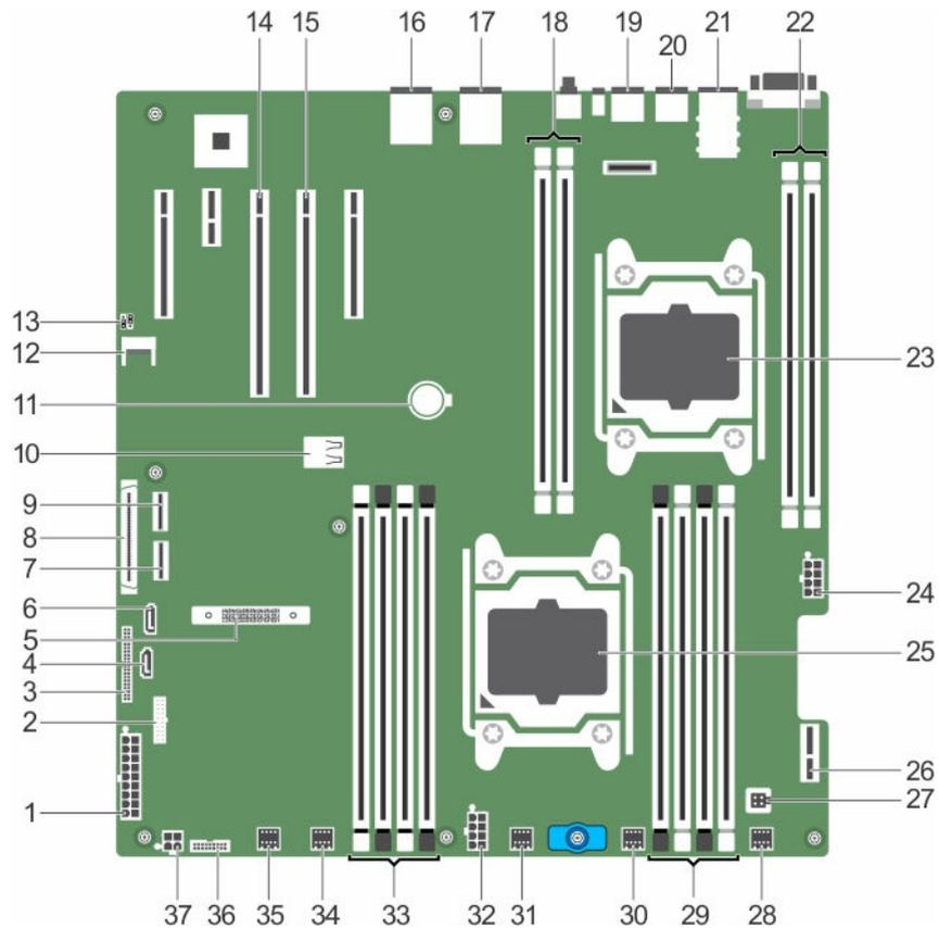
Figure 60. System board jumpers and connectors
