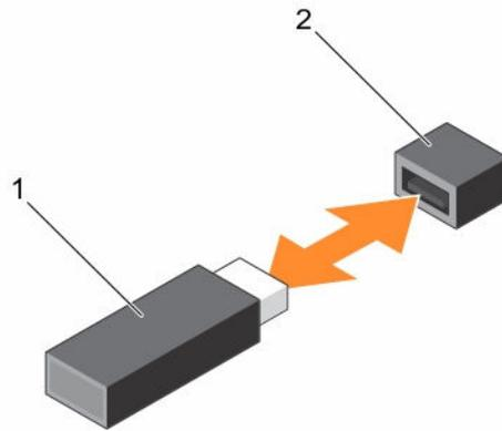
**Figure 30. Replacing the internal USB key**
