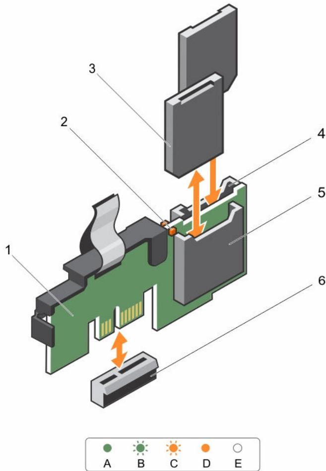
**Figure 35. Removing and installing the Internal Dual SD Module (IDSDM)**
