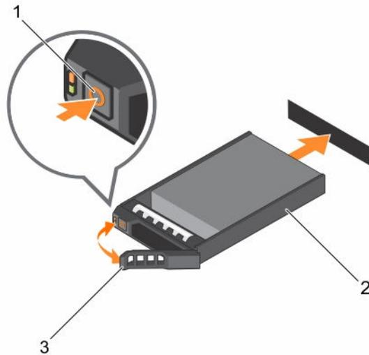
**Figure 23. Removing and installing a hot-swap hard drive**
