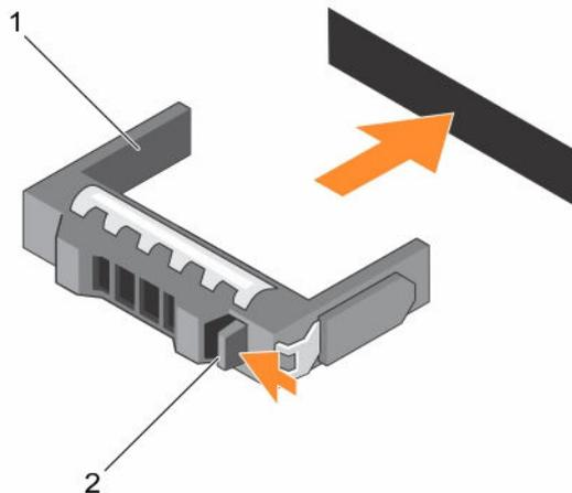
Figure 21. Removing and installing a 3.5 inch hard-drive blank
