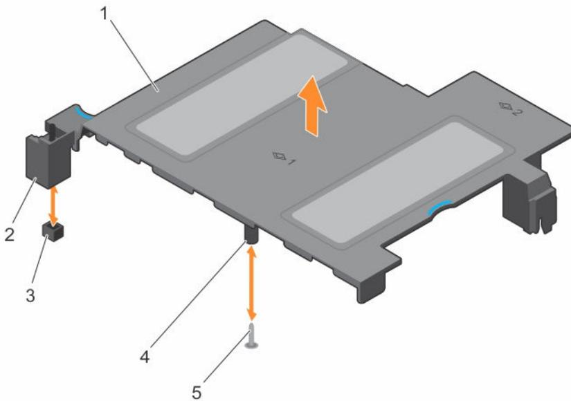
**Figure 16. Removing and installing the cooling shroud**
