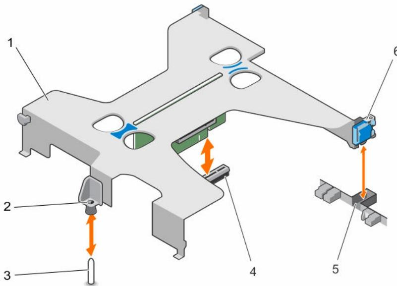
**Figure 31. Removing and installing the expansion-card riser**
