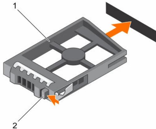
**Figure 20. Removing and installing a 2.5 inch hard-drive blank**
