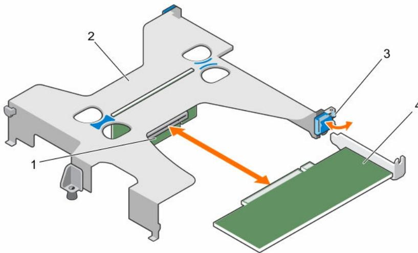
**Figure 32. Removing and installing the expansion card from expansion-card riser**
